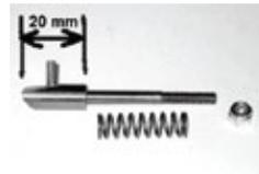
**P351** Polar False Clamp Latch Pin Assembly. Fits Polar 92, 115, 137 and 155 ED, X, XT and XS models. Fits all 78 models. Measures approximately 60mm (2.375") long. The main latch area is 8mm in diameter by 20mm long. Includes latch pin (232333), perpendicular dowel pin (201558), spring (205687) and self locking hex nut (201091).
