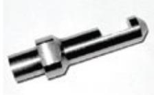
**P11** False clamp pin for the later models of Polar cutters after approximately 1984. Measures 7.75mm in diameter X 40mm (1.58") long, notched as shown. (232338)
