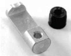
**P210** Polar slider or push pin. This slider was originally made of black plastic. Ours is made of aluminum. Measures 9.5mm (.375") in diameter X 25.5mm (1") long. It is used to release the false clamp latch pin. Equal to Polar 241828. Does not fit the Polar 155 and 176 models. Comes with a black pastic hole plug. Polar part #241827.
