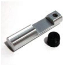
**P220** Polar slider or push pin. this slider was originally made of black plastic. Ours is made of aluminum. Measures 9.5mm (.375") in diameter X 42mm (1.625") long. It is used to release the flase clamp latch pin. Equal to Polar #241829. Only fits the Polar 155 and 176 models. Comes with a plastic hole plug. Polar part #241827.
