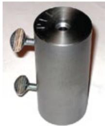
**FPA25** False clamp pin installation tool. This steel anvil tool is 1.750" in diameter by 4" long. It is used to position and hold the Polar false clamp pin in place while the bottom end of the pin is peened over with a hammer. One end is machines to fit over the P10 pin while the opposite end fits over the P11 pin.
