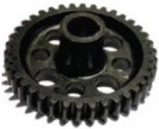
**G338** Polar Lead Screw Gear, Equal to Polar 224231. This black plastic gear has 38 teeth and measures approximately 100mm (3.938") in diameter by 14.7mm (.563") wide at the gear teeth. It has a 19mm (.750") diameter bore with a 6mm wide keyway. Fits Polar 76EM up to machine serial #5761301, Polar 92 EMC and Polar 92 EMC MON models up to serial #5711301, Polar 92 s, Polar 92 E, Polar 92 EM, Polar 92 ED, Polar 92 X and Polar 92 XT up to serial #6511201.
