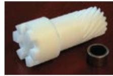
**G325** Pinion Gear for Polar hand fine adjustment mechanism. Machined from Delrin plastic. Supplied with internal needle bearing. 15 helix teeth. (206286)
