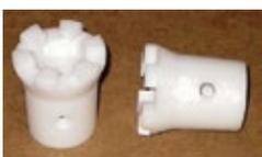
**G324** Polar Claw Clutch Gear, equivalent to Polar number 206292. This 6 lugged "gear" engages out part number G325, the Polar hand fine adjusting gear. It is used in the backgauge hand fine adjustment mechanism on many Polar EL, ST and CE cutters, such as the 71 & 72 models (before machine serial number (4551001), 90 CE, 115 CE (before machine serial number 4431931), 150 and 155 CE cutters. It measures 1.250" in diameter at the claw tooth end by 1.375" long.
