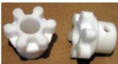
**G320** Hand Fine Pinon Gear (equivalent to Polar 218628.) This 6 tooth gear is used in the hand fine adjustment mechanism on some early Polar EL and Polar CE paper cutters. Measures 1.47" (37mm) in diameter over the 6" teeth. Overall length is approximately 1.062" (27mm) long. It has a 14mm bore and is drilled for a roll pin.
