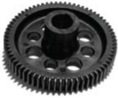
**G335** Polar Lead Screw Gear, equivalent to Polar #245010. It has 68 teeth and is approximately 105mm (4.125") in diameter. It measures 15mm (.563") wide at the teeth. Has a 19mm (.750" diameter bore with a 6mm wide keyway. Fits 76 EM cutters after serial #5761301 and 78 and 92 cutters after serial number 6511201.
