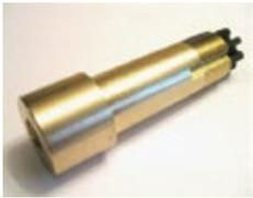
**G314** Polar Pinion Gear Kit equal to Polar 059882, 044924 and 256969. This kit is Polar original part #059882. Includes the brass pinion gear (044924 or 256969), washers (202843, 222745, 220951, 022332), screws (202080, 201566), 2 black plastic gibs (221894) and white plastic backing plate (026634). The gear measures approximately 25.2mm (.98") in diameter at the large end by 85mm (3.35") long. There are 7 gear teeth at the back end and there is an 8mm hex socket at the front end.
