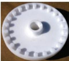
**G321** Hand Fine Spur Gear (equivalent to Polar 218629). This 22 tooth gear is used in the hand fine adjustment mechanism on some of the early Polar EL and Polar CE paper cutters. Outside diameter of 4.97" (126mm). Overall width is approximately 1.57" (40mm). It has a 19mm diameter bore (.75") and a 6mm wide keyway.
