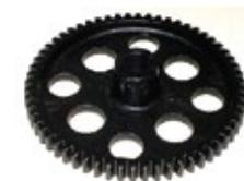
**G329** Polar Lead Screw Gear equivalent to Polar 222205 (ZA3.222205). This black plastic gear has 60 teeth and measures approximately 155mm (6.125") in diameter by 14.8mm (.583") wide at the gear teeth. It has a 19mm (.750") diameter bore with a 6mm wide keyway. Used on Polar 115 EMC and 115 EM (up to machine serial #5731401), 137 EMC (before machine serial #5721001). This does NOT fit any Polar Autotrim models. This does NOT fit and Polar 58, 76, 78 or 92 models.
