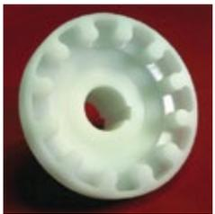
**G319** Hand Fine Spur Gear (equivalent to Polar 218631). This 12 tooth gear is used in the backgauge hand fine adjustment mechanism on Polar 72 EL, 72 CE and PM cutters, after machine serial number 4551001. Outside diameter is 2.97" (75.5mm). It's overall width is approximately 1.57" (40mm). 19mm diameter bore and 6mm wide keyway.
