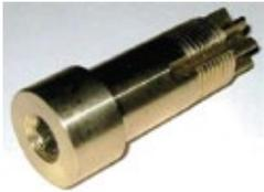
**G315** Polar Pinion Knife Change Gear 014628, 245954. This bronze pinion or "gear" is used in the blade carrier during blade changes. It measures 25mm (.98") in diameter at the large end by 65mm (2.56") long. There are 7 gear teeth at the back end and there is an 8mm hex socket at the front end.
