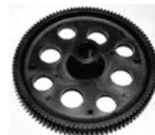
**G330** Polar Lead Screw Gear, equivalent to Polar 245004. Black plastic gear has 106 teeth, measures approximately 162mm (6.375") in diameter by 15mm (.583") wide at the gear teeth. Has a 19mm (.750" bore with a 6mm wide keyway).
