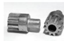
**G331** Polar Fine Adjustment Gear, Polar part #245078. This cast aluminum handfine gear has 11 teeth and measures approximately 19.5mm (.77") in diameter by 34mm (1.34") long. Requires drilling during assembly. Supplied with new spring pin.
