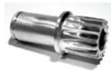
**G327** Polar Track Change Gear. Used on Polar 115 CE and Polar 155 CE cutters built during the 1970's. The gear is used in the mechanism which changes the "track" on the wide magnetic tape on cutters with the magnetic tape program storage system. This 15 tooth gear is machined from aluminum and is a direct replacement for the metal and plastic original gear. (010591)
