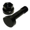
**S102** Alloy steel shear pin complete with washer faced hex nut (231661). The head is 1.180" diameter X .39" thick. A flat on the head is provided as shown. The shank is 2.330" long below the head and has a 16 mm thread.
