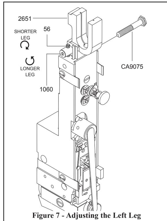
Figure 7 - Adjusting the Left Leg
