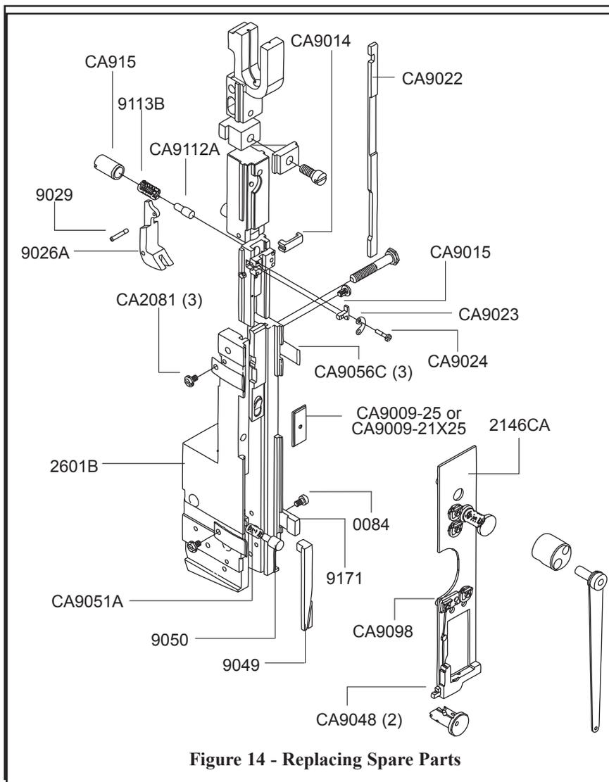
Figure 14 - Replacing Spare Parts
