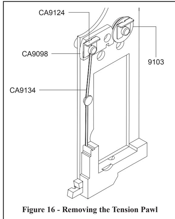
**Figure 16 - Removing the Tension Pawl**
