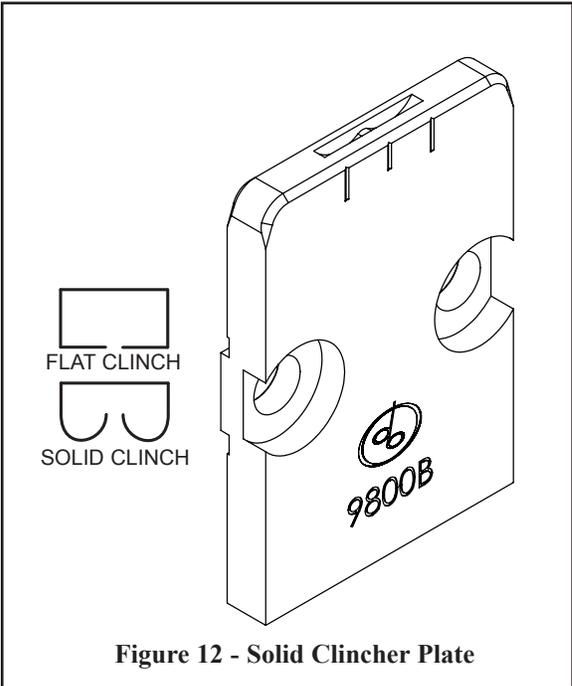
**Figure 12 - Solid Clincher Plate**
