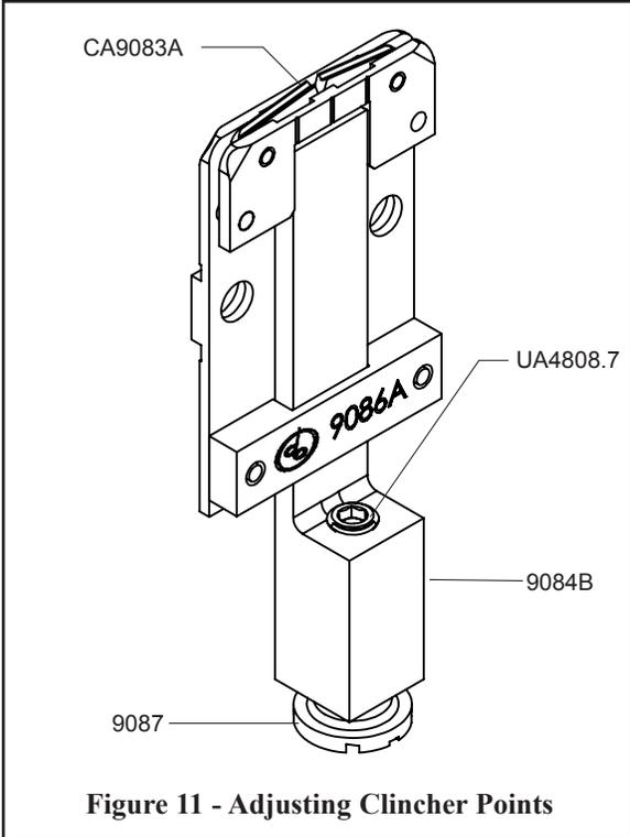
**Figure 11 - Adjusting Clincher Points**
