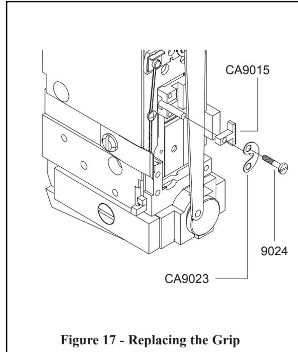
Figure 17 - Replacing the Grip
