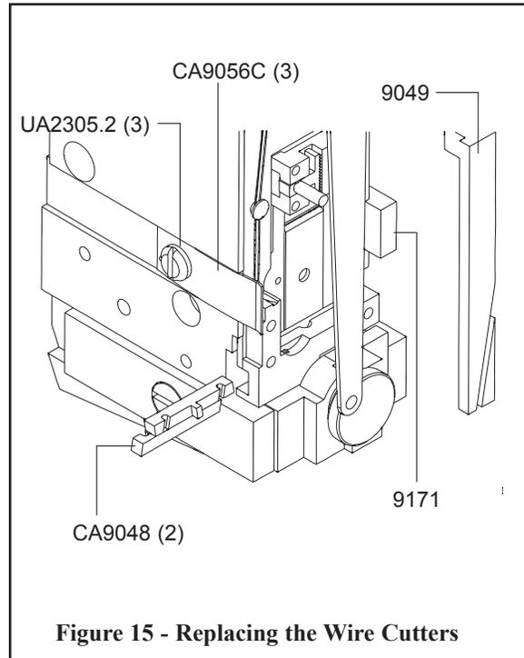
**Figure 15 - Replacing the Wire Cutters**
