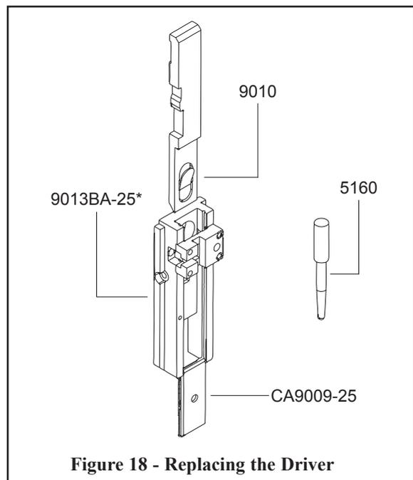
Figure 18 - Replacing the Driver
