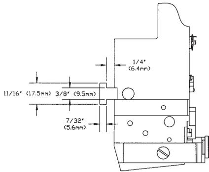
\*T-SLOT FOR ADJUSTABLE AND GAND MOUNTING OF HEADS
